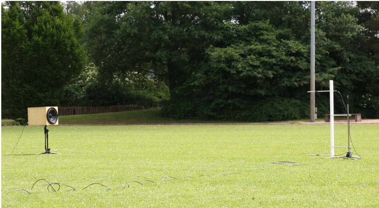
Figure 3: Measuring the surface impedance of a lawn with the transfer function method with two vertically separated microphones.
